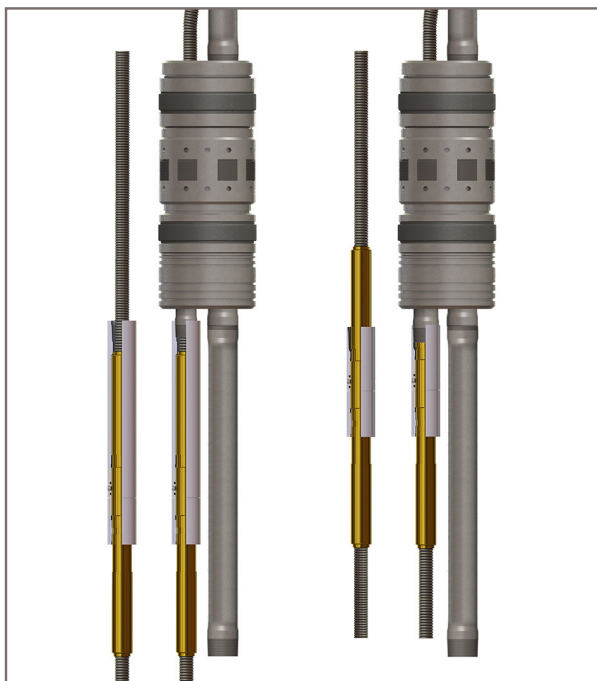
EA1504 Crossover shown below the packer, and as a cut-away view. Assembly on left is shown installed in a small secondary bore. ESP cable can be supplied with factory molded MLE to avoid splicing below the packer.
